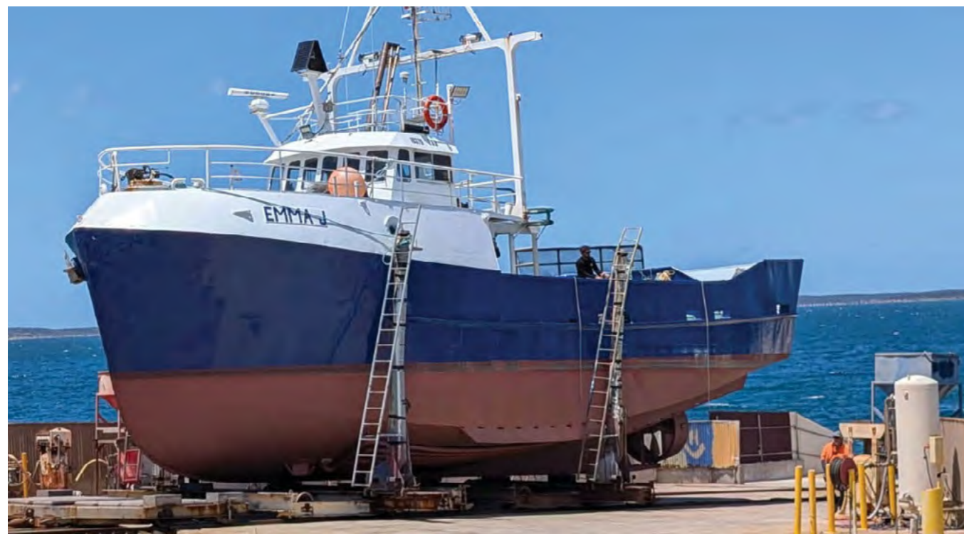
Former pilchard purse-seiner Emma J undergoing conversion to a coral trout mother ship.
