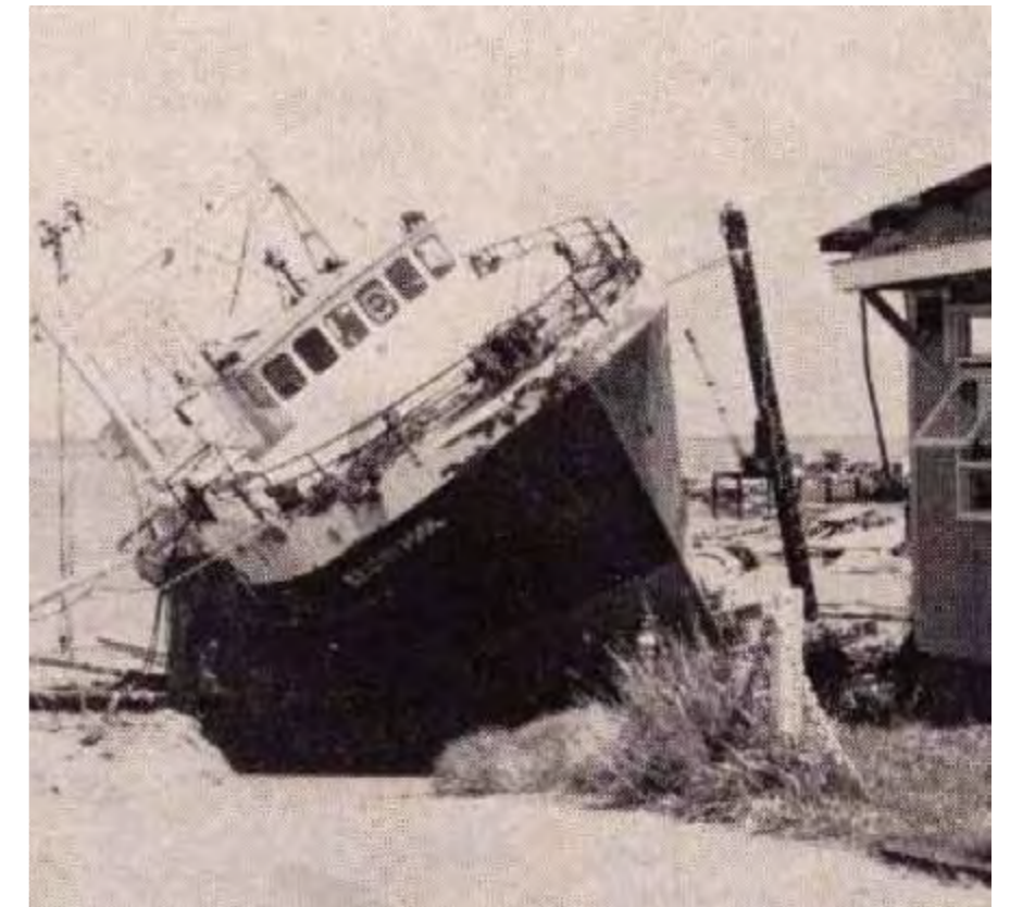
The 23-metre trawler NR Liverpool lying on its side after being blown off a cradle at the small ships slipway in Darwin during Cyclone Tracy. (Photo: Royal Australian Navy.)
